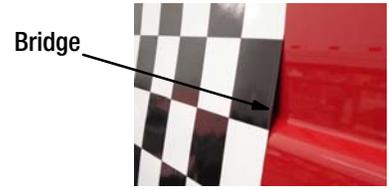
3. **For film IJ380:** Start with the heat gun set to 250°F and heat the film (step 4) to 120-130°F (50-55°C) for convex and concave areas including bumpers and channels.
